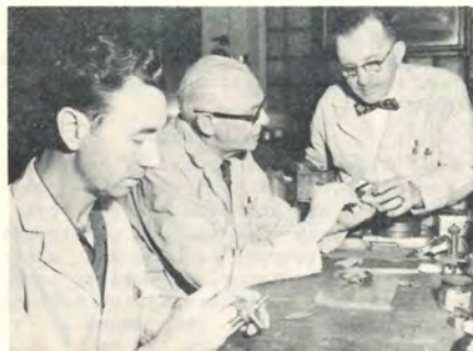
The men pictured above, Don Materdomini, James Dipp, and James Pennachio, Shop Foreman of the Machine Shop, Tech Main, are in the process of repairing film cleaning squeegee to be used in motion picture developing machines, to be installed in the Motion Picture Laboratory at the Center.
