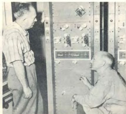
John Jorgensen (standing) and Frederick Frintrup are putting the finishing touch on two newly acquired 35mm Magnetic Recorders to be used in the sound recording room. The new recorders can record and play back, whereas the old ones could not. The two machines above will replace six of the "primitive" types, of which three are still in use.
